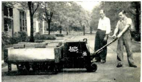
New Hydroelectric Lift Truck being tested by Howard Atteberry. Ed Stille looks on.
