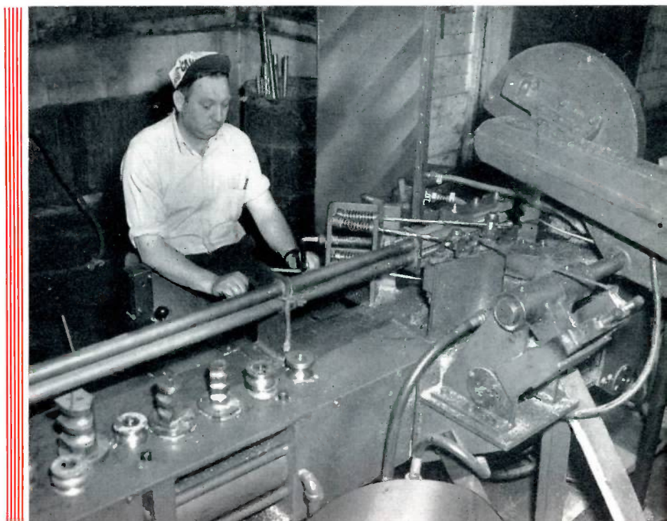
Above, William Currie is boring a 45° wrought copper elbow. He has been with Mueller six years. Below, George Fcslett, a ten-year employee, operates the rod tube bender which forms the 45° and 90° elbows from copper tubing.
