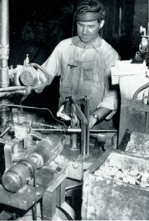
Above, William Currie is boring a 45° wrought copper elbow. He has been with Mueller six years. Below, George Fcslett, a ten-year employee, operates the rod tube bender which forms the 45° and 90° elbows from copper tubing.
