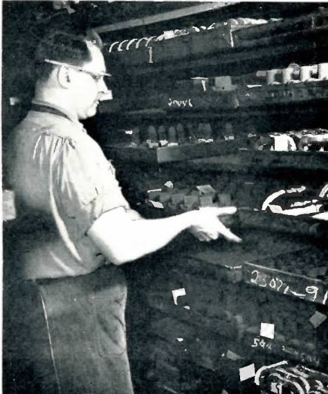
Core storage provides a readily available supply of cores to meet the foundry demand.
