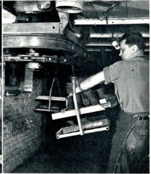
Lois Harper, core cleaner and inspector, starts a pan of cores on their trip via conveyor to the brass foundry. Across the street, Earl Lewis, core storage handler, lifts off another newly arrived pan which is placed in storage until the cores are required in the foundry.
