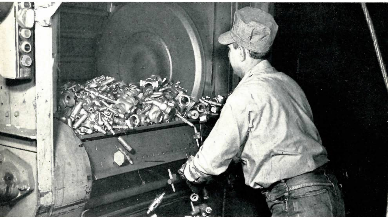
Castings are first cleaned in a wheelabrator, which removes cores and molding sand. Here Gerald Sarver empties castings from wheelabrator barrel to hopper for transfer to the "water rattler."
