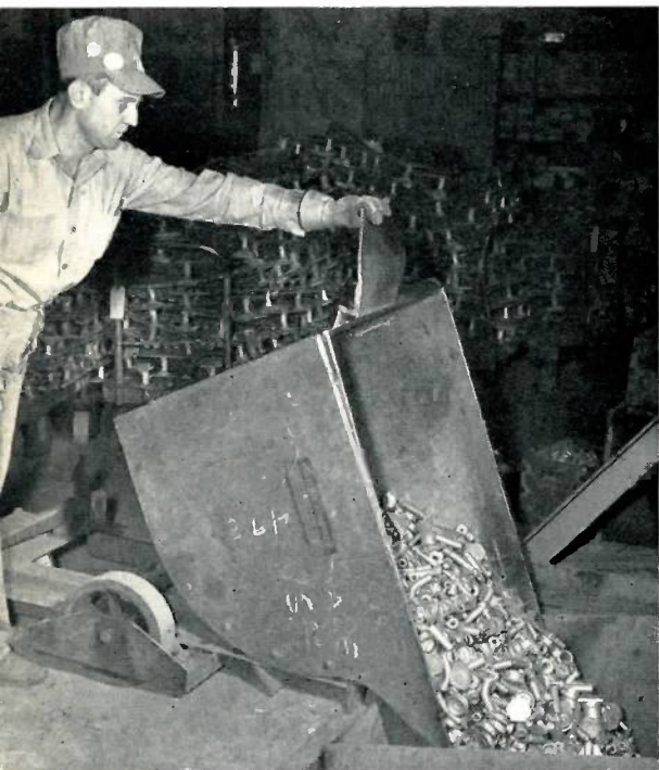
Mixed castings are loaded into the "water rattler" for washing and polishing operation.
