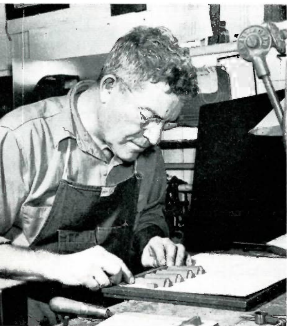
Lester Skelley, the pattern shop's oldest employee, makes a layout on paper for a master pattern.
