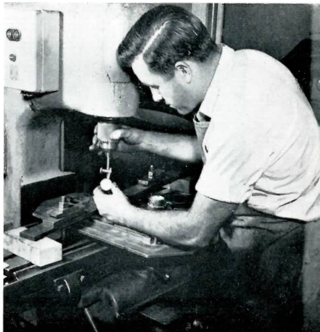
Royal Skelley is shown repairing a pattern for a regulator. He is making a check for concentricity.
