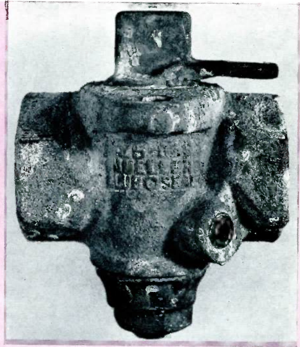
Burned LUBOSEAL which went through series of tests.
