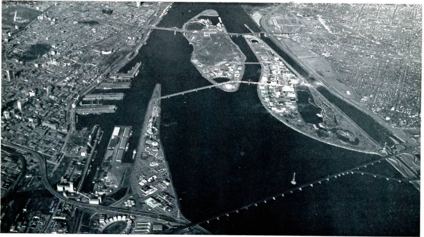
Much of the 1,000 acre site is man-made. Nearly 30 million tons of fill were used to enlarge the existing island park of Ile St.
