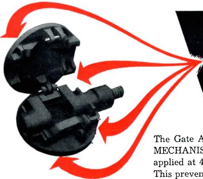
The Gate Assembly contains the 4 POINT WEDGING MECHANISM. When the valve is closed, pressure is applied at 4 POINTS near the outer edges of the discs. This prevents warped or sprung discs and prevents any chance of leaking. Before you replace any old valves or install new ones, be sure you know all about this superior Mueller Gate Valve. Write us for full information.
