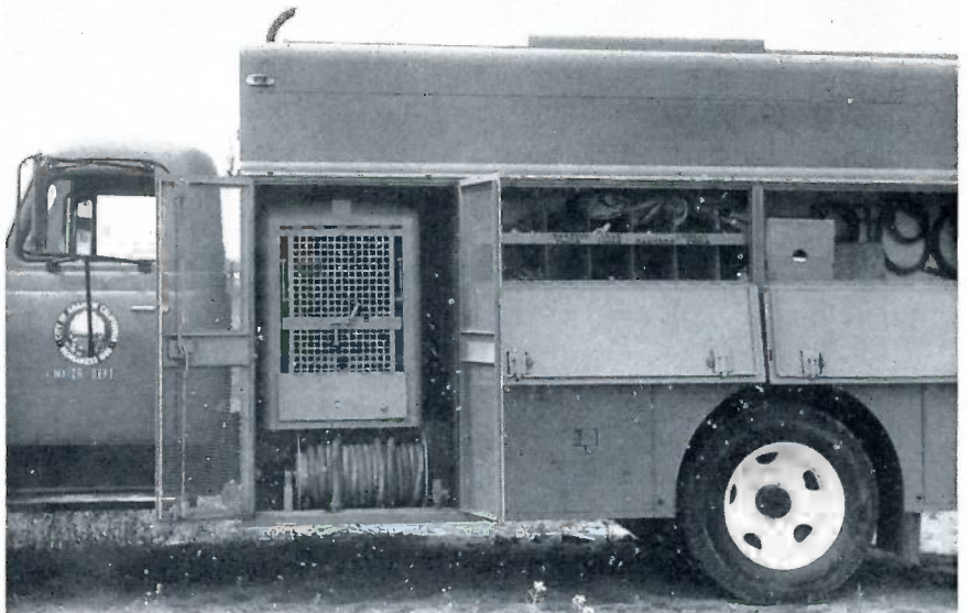
Overall view of left side of the Service and Heavy Construction Unit, showing tool compartments and compressor motor.
