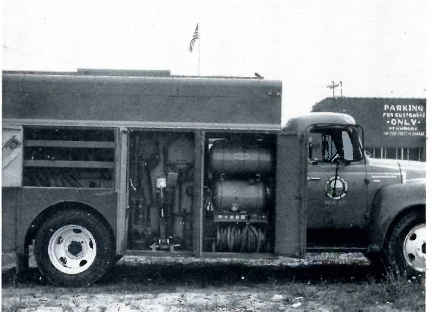
Overall view of right side of the Service and Heavy Construction Unit, showing compressor tanks, large pneumatic tools, and more small tool compartments.
