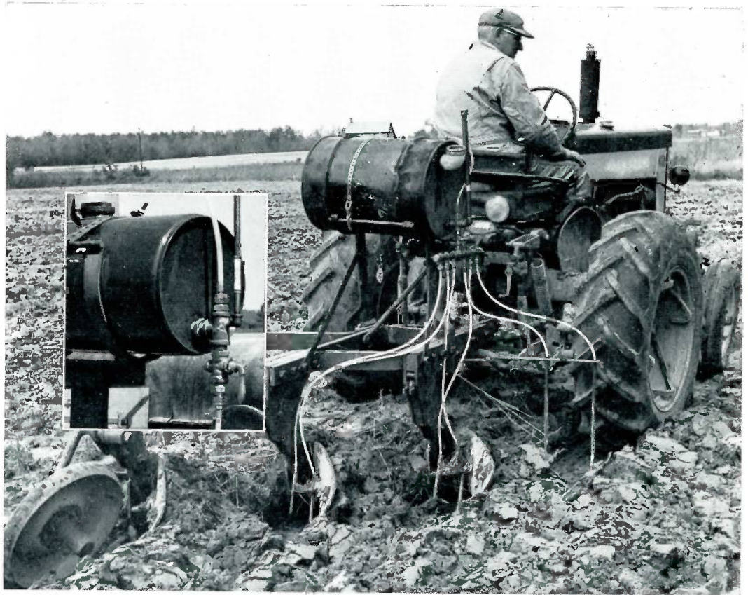
Mueller gas stops are shown at work as a means of control for soil fumigants.
