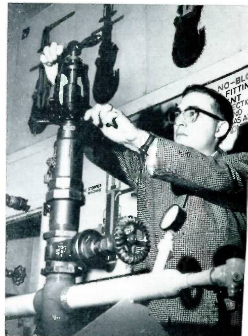
One of the "students" operates some Mueller line stopping equipment on a mock-up line after Mr. Sheerer completed his instruction and demonstration in the lower photo.
