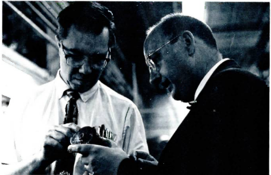
In the upper photo, Mueller Co.'s Manager of Quality Control Elmer Fawley takes a close look at the key port of an ORISEAL valve that recently finished 110,000 cycles at Frankfort, Kentucky. In the lower photo, Carl Floren, group project engineer, and William L. Hauffe (right), senior project engineer, examine the part for unusual wear.
