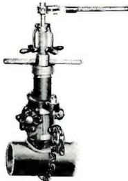
article possessing requisite strength and provided a thread which insures a thoroughly dependable connection of brass corporation cock with the iron main.
