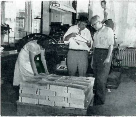
Jim Clay, plant superintendent, and Ed Clauder, bindery foreman, check the fold of 32 pages of the Mueller catalog as it comes off the folding machine behind them. The folding machine creases 32 pages at one time.
