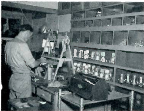
A corner of the shop where meters are tested and kept in repair. There are more than 15,000 meters serving the Monterey Peninsula.
