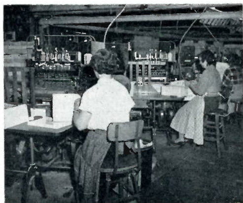
Girls in the sewing machine row in the bindery are sewing the various signatures of the Mueller catalog together to form a complete book. (A signature is a folded printed press sheet.)
