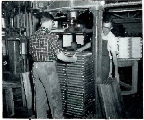
Craftsmen are placing stacks of Mueller catalogs in the hydraulic book press. Pressure is applied and the catalogs are left to "set" overnight. This sets the glue.
