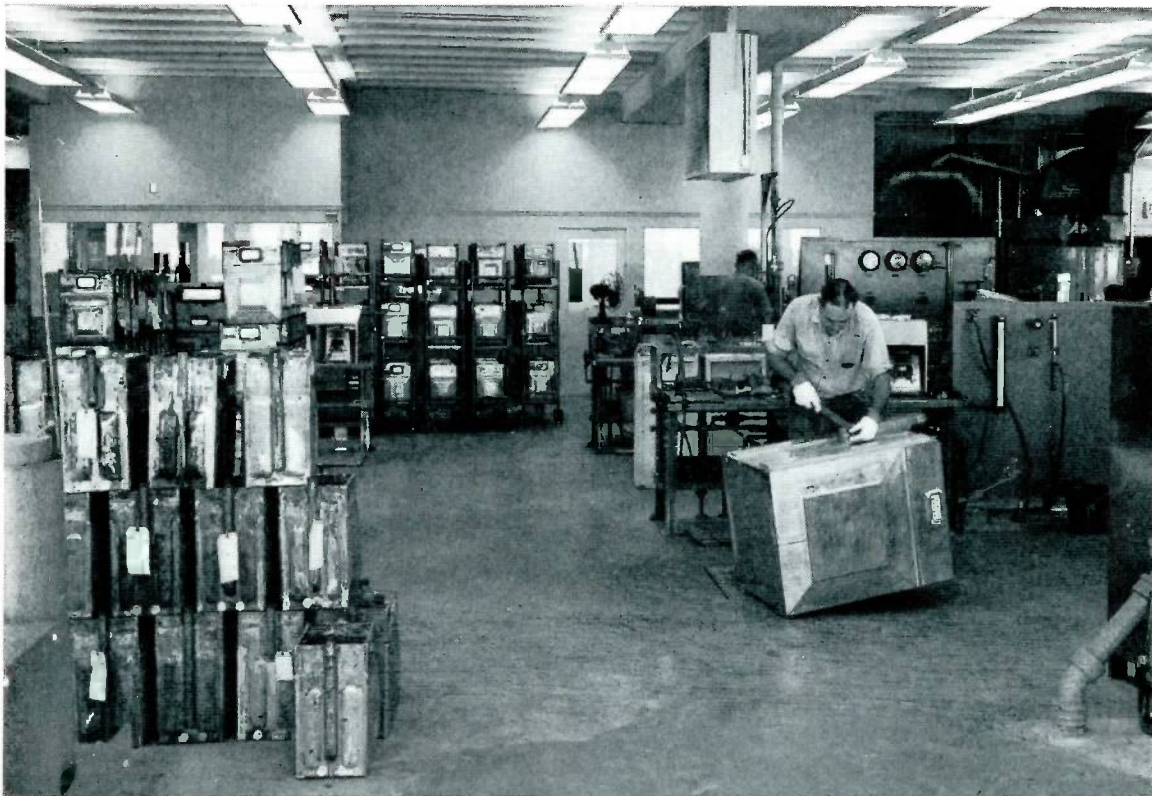
Repaired meters are loaded on the conveyor which takes them through a degreasing unit (center) to a paint booth (right) where they are sprayed. Each meter makes three
