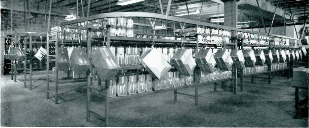
After final spraying a conveyor carries the newly painted meters into the storage area where they are kept in stock. The conveyor runs between the spray room and the
