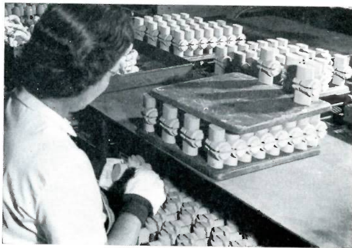
Each core produced is individually cleaned and inspected before it goes to the foundry.
