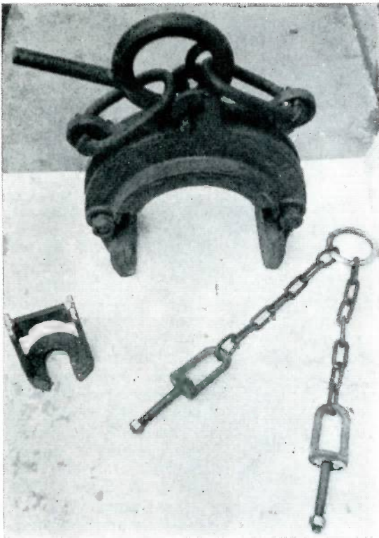
The simplicity of the two devices designed for handling valves and hydrants is shown in this close-up. The tool for handling valves is above at the left and the hydrant handler is on the right.
