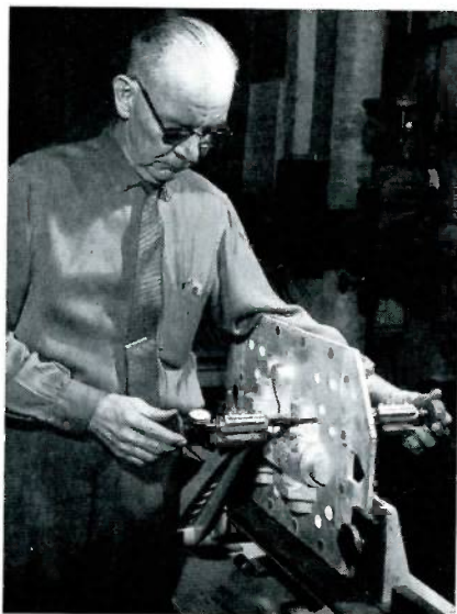
Without an exacting pattern to start with, most castings would be incorrect. Pattern Shop Foreman Ollie Fortschneider checks the alignment of a pattern to be sure that it is without .001 of an inch.
