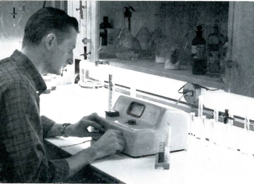
Analysis of foundry metals is continually being carried out. Lab Technician Maury Sefton checks the nickel content of brass on a spectrophotometer.
