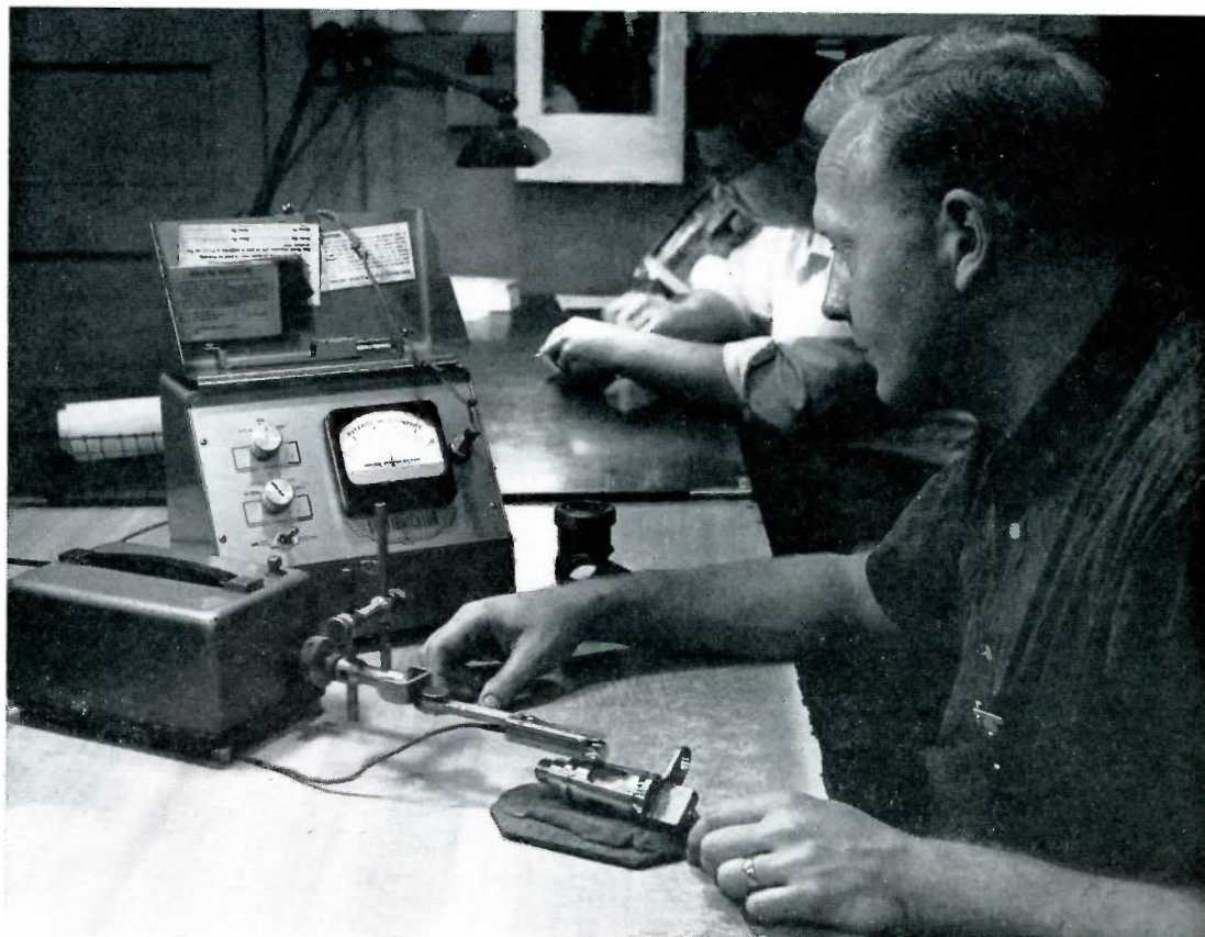
Precision parts can't be produced without precision tools. Toolmaker Bill Brunner projects a magnified image of the tool on a screen to check if the exact angle is cut into the tool. This contour projector is able to magnify a tool up to 62\frac{1}{2} times. In other words, every 16th of an inch on the screen is equivalent to a thousandth of an inch on the tool.
