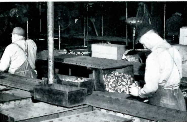
Once the rough castings have been cleaned, inspectors check each one before it goes on to the grinding and machining processes.
