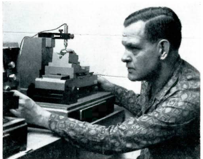
Lindle (Hap) Hockman, Test Lab Lead Man, checks a key on a machine that is able to detect a surface flaw that is no greater than one millionth of an inch. The model shop or machine shop, (below) which is an intricate part of the lab, produces prototypes and makes modifications of products under test and development.
