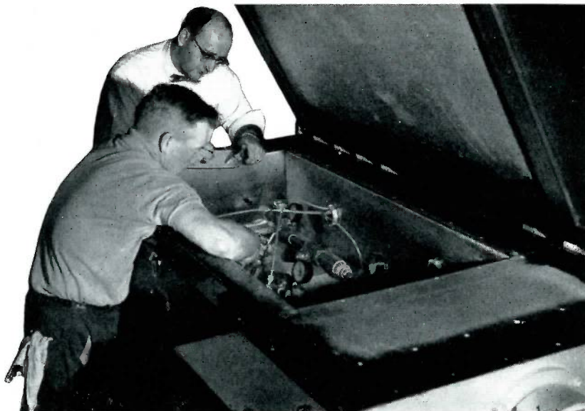
Mueller products are tested under pressure in this "deep freeze" that is capable of dropping temperatures to a minus 60 degrees. Test Lab Operator William Hood (foreground) checks the turning torque on some stops as Project Engineer William Hauffe records the data.
