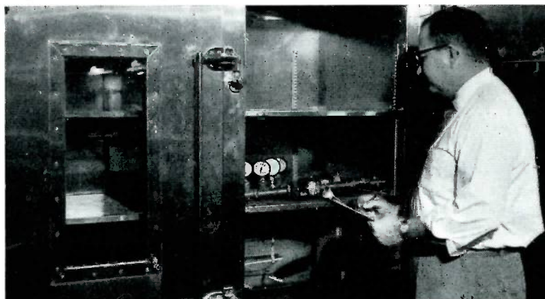
George F. Binkley, Manager of Engineering Services, (above) checks readings in a humidity cabinet while (below) Assistant Project Engineer Paul R. Ammann removes some valves from the test oven where temperatures of 600 degrees can be produced.
