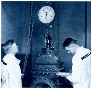
The weight and dimensions of each part and the assembled valve are carefully checked and recorded.
