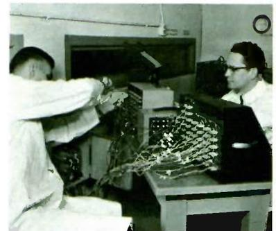
Strain gages are wired, calibrated and connected to precision electronic recording equipment.
