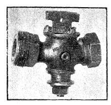
D-22000. The roller passed over the box, pressing down the standpipe, and the rod forced the key down 3%" through the body.
