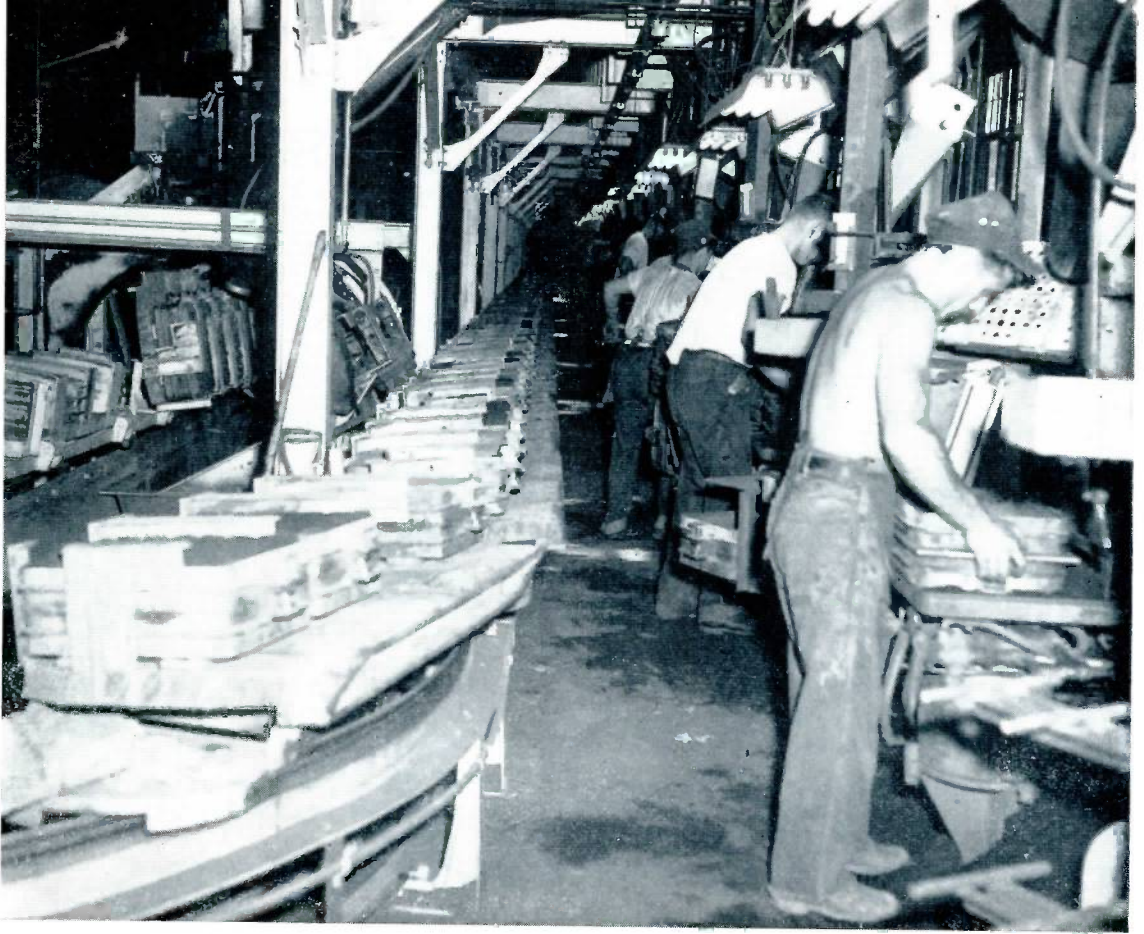
Visible above are a part of our Plant 4 machine molders each of whom makes molds and places them on the individual cars of the train. To maintain a high rate of production, four trains are in constant operation. While molds are being placed on one train, they are being poured in the second. The third is in a cooling section and the fourth is going through the shake out area where sand and castings are shaken from the flasks. Note the train of molds being dumped in the background.
