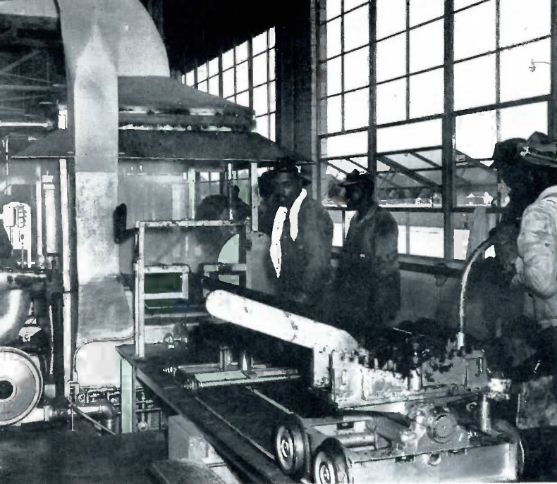
The photos on this page were taken in the pipe-coating and wrapping plant. Here you see small pipe being coated and wrapped for protection.
