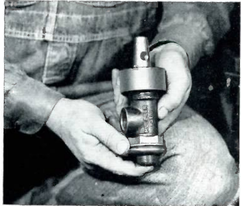
5. Built-in valve of tee is closed and tee threaded in easy-release screw plug, which now replaces the combined drill and tap on the boring bar of the B machine.
