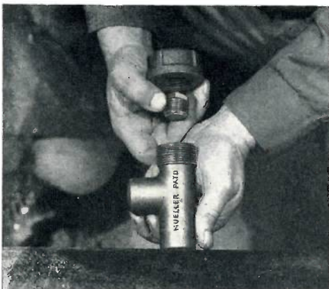
1. These parts comprise the Mueller welding tee: cap, bronze plug and forged steel body.
