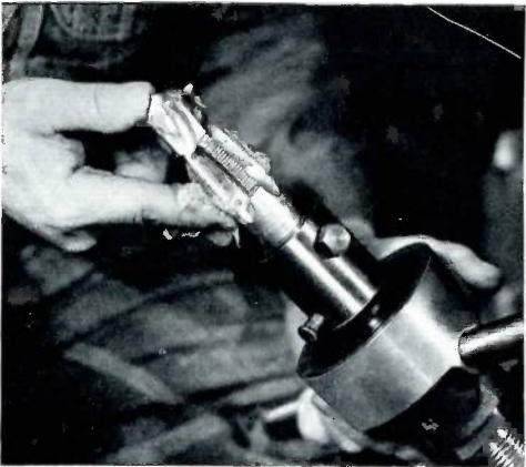
3. Before inserting the combined drill and tap in the machine, it should be coated with Mueller cutting grease for easier operation and to prolong life of tool's cutting edges.
