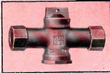
Inverted key curb stop with long Dresser Coupling Ends, Style 90. (Especially designed for installing in a line without a curb stop or to replace existing curb stops.)
