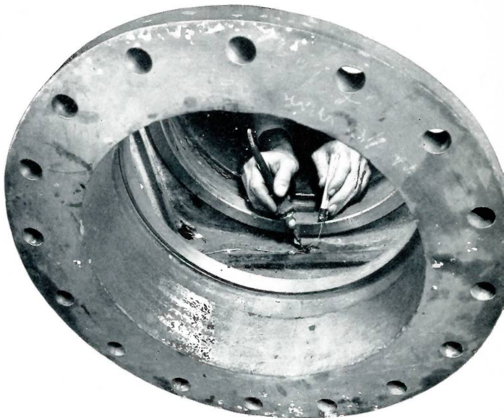
The tiny hair-like wires of the strain gauge are attached to heavier wires which are being soldered in place by the lab operator.
