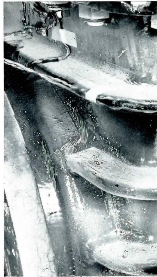
The white lines on the body of the valve are cracks in the stress coat material.
