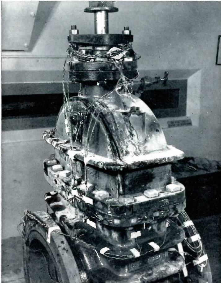
The extreme water pressures in the valve caused the crack in the bonnet which can be seen clearly in this photo. Even though the valve is ruptured the test does not end here. Further investigation continues to determine why the valve cracked at this point.
