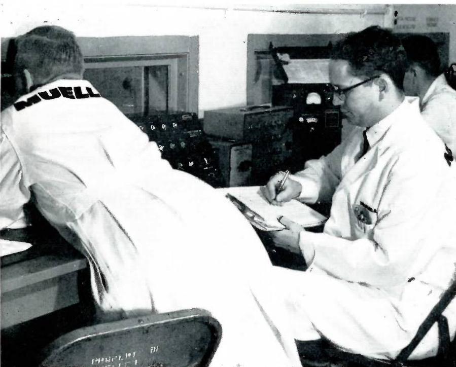
This is the scene in the control room as the test gets underway. The valve is observed through binoculars while gauges, amplifiers and recorders chart changes in the valve as water pressures change.
