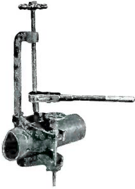
The Crow and Ratchet Method of Tapping Water Mains
