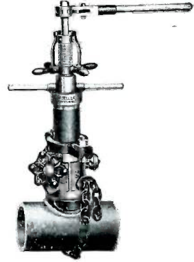
Mueller machine furnishes modern way of tapping
