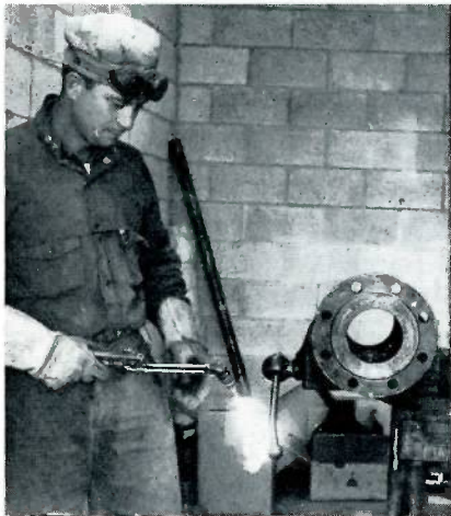
James W. Grant, welder, gets ready to work on flange for large volume meter installation in Center's welding shop.
