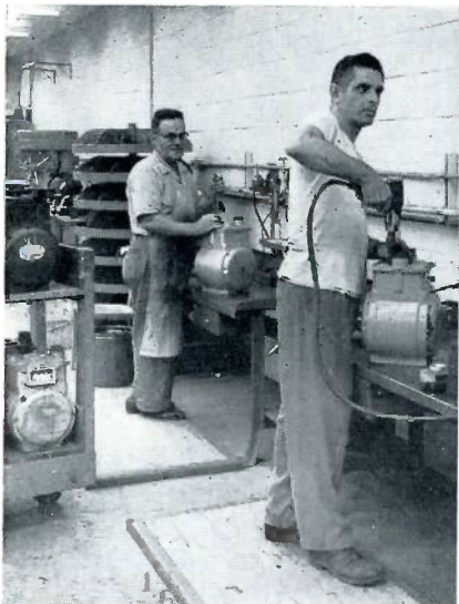
Large meter shop has bench where Leslie Littral, left, and Raymond Wilson repair 240 iron case meters monthly.
