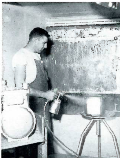
New Center feature is paint booth with water carrying off paint as Billy Edwards, meter repairman, sprays meters.
