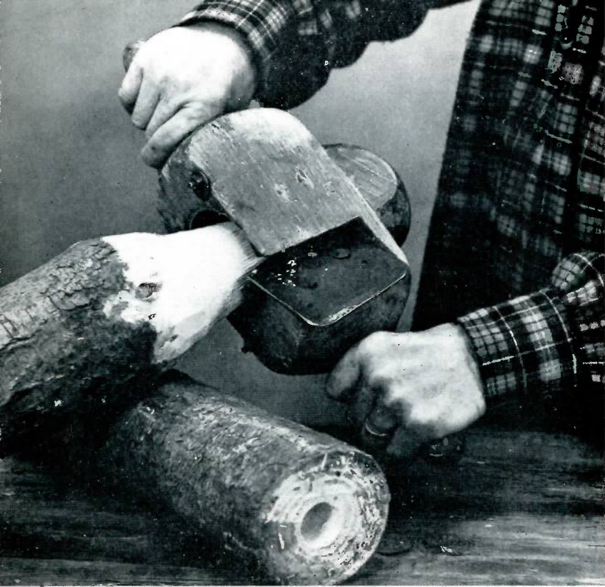
After a log is bored, one end of the section is tapered with a tool made from a hardwood block and a hand forged blade.
