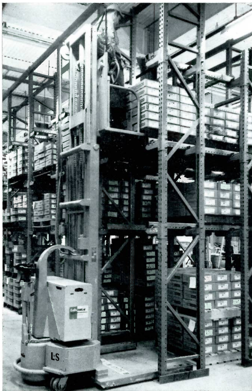
This remote controlled order picker was recently put into use at Mueller Co. in Decatur as part of an overall effort to speed service and shipments to customers.
