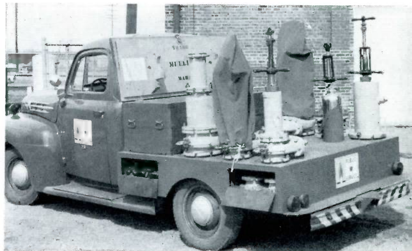
These side panels house tools, adapters and fittings which are always on the truck and ready for immediate use in case an emergency arises.
