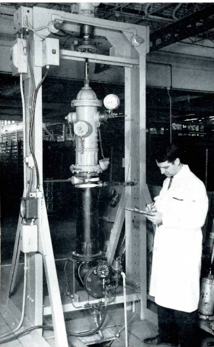
Hundreds of hours of tests confirmed the calculations of Mueller engineers. Performance and long-lasting dependability of the operating mechanism, main valve and drain valves were proved by continuous operating cycle tests (left). Carefully metered flow tests (below) were conducted to prove the maximum flow capability and full flow performance of the shoe, main valve, barrel and nozzle waterway.
