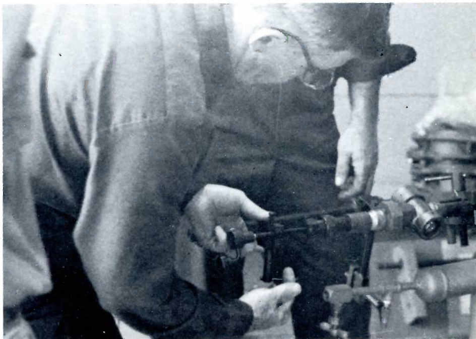
Utility men look on as Bill Knorr prepares to assemble an insertion machine to a small line stopper fitting. Later the men will use the equipment themselves.
