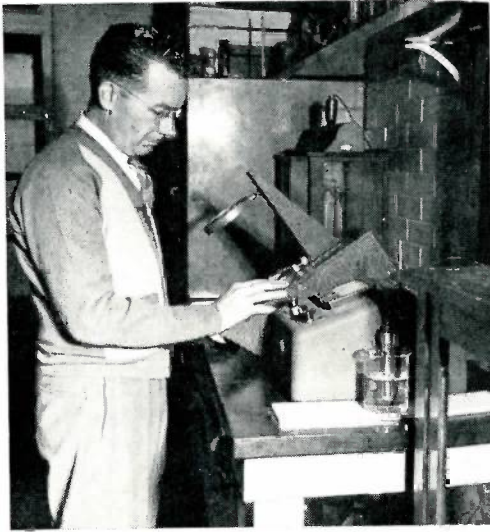
Most important factor in safeguarding purity of water is the constant check made by local authorities. Here Gerald Davis, Decatur city chemist, makes a bacteriological plate count.
