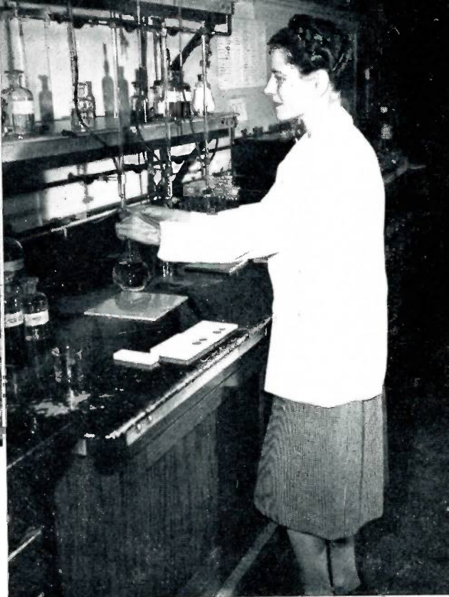
Linda Marsh, chemist, titrates the alkalinity of a sample of water. This is one of the routine chemical tests made in the analysis of water.
