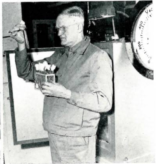
Frank Turner, chemist at the Paris, Illinois, water works, examines lactose fermentation tubes for presence of gas, a presumptive test for E. coli , an organism indicating pollution.
