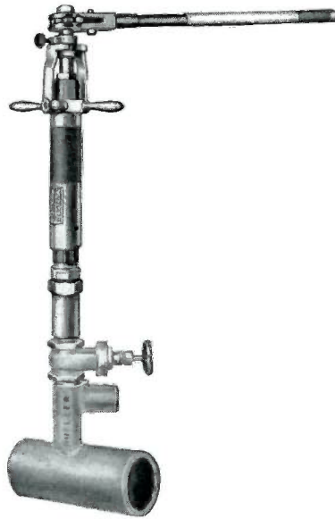
Mueller "D-4" Drilling & Inserting Machine Capacity 1" to 2" Inclusive
