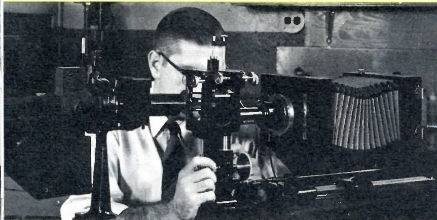
The microstructure of raw materials and metal in products are inspected under extreme magnification in the metallograph.
