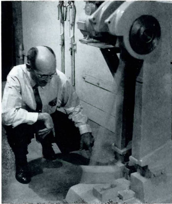
A cold chisel is in the midst of receiving the "beating of its life" as this calibrated machine hammers away under the watchful eye of Project Engineer Wallace Gould.
