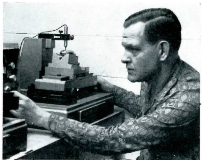
Lindle (Hap) Hockman, Test Lab Leadman, checks a key on a machine that is able to detect a surface flaw that is no greater than one millionth of an inch. The model shop or machine shop, (below) which is an integral part of the lab, produces prototypes and makes modifications of products under test and development.
