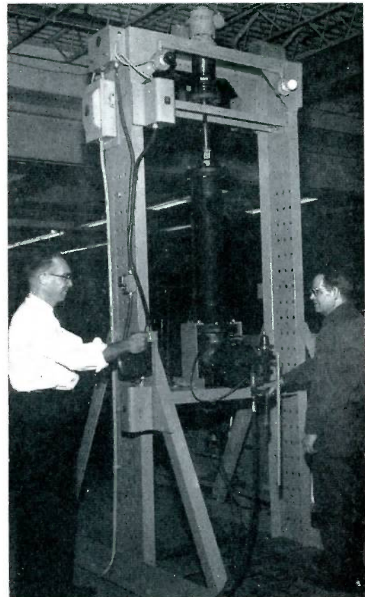
This cycling machine opened and closed this fire hydrant part thousands of times during just one test. John J. Smith, Chief Products Engineer, checks the counter while Operator Louis Bland checks the water pressure.
