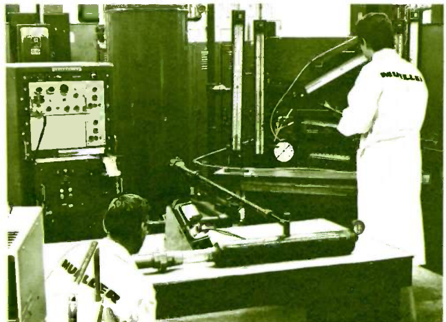
Flow testing of a simulated installation to determine the effects of line debris on flow performance.
