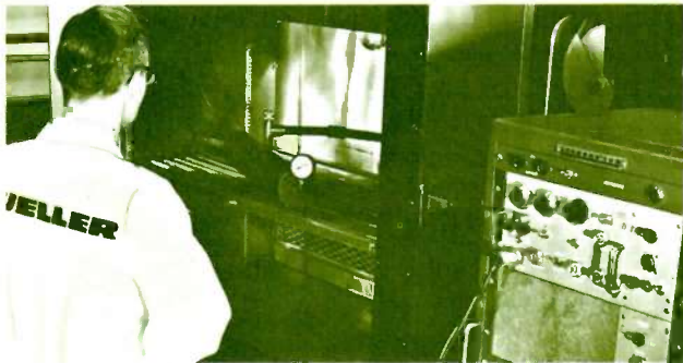
Testing to determine the effects of low temperature on flow performance.
