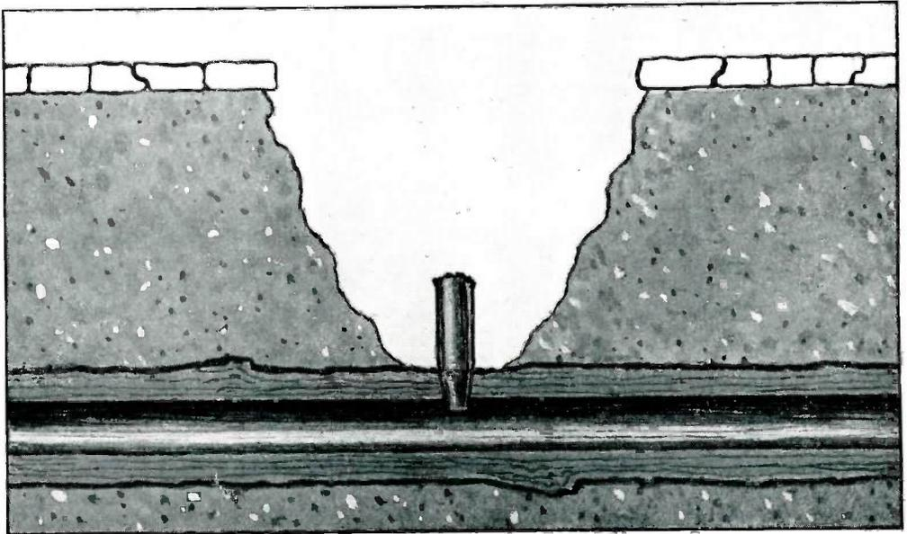
*Fire hydrants are still called "fire plugs," a carry-over from the days of wooden mains and iron men. A water supply is the first requirement for fire-fighting, and in the early days it was necessary to dig down to the main and drill into it. After the fire had been extinguished, a wooden plug was driven into the main to prevent any further loss of water.*
