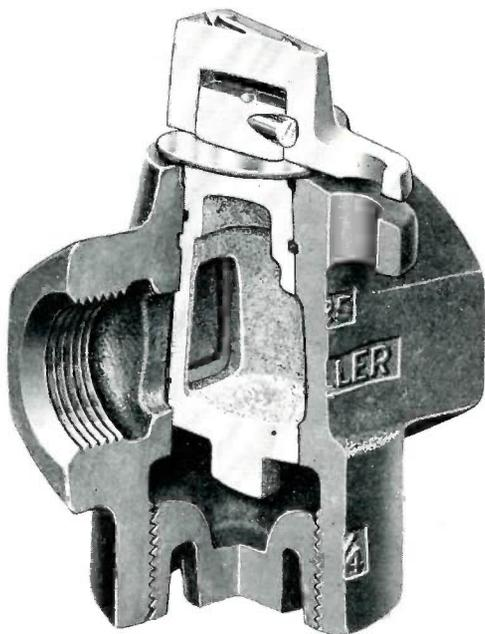
*This sectional view of the H-11112 gas meter stop shows its rugged construction. Details shown include the permanently pinned head, the heavy gray iron body, the stop's inverted key, and the special lubricating plug.*
