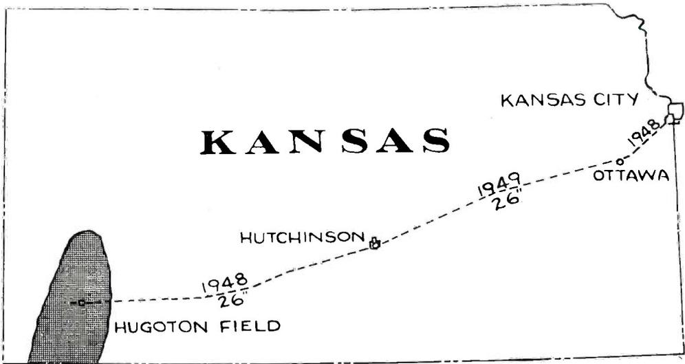
*Route of Cities Service Gas Company's new 26-inch pipe line is shown on this map. Two links in the line will be completed in 1948, the third and final section, between Hutchinson and Ottawa, in 1949. The cross-Kansas line will increase gas available to the Greater Kansas City area in excess of 50 per cent. Estimated cost of the line: 25 to 30 million dollars.*
