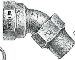
Inlet—MUELLER Thread Outlet — For Copper Service Pipe with Straight Coupling Nut. (Gasket Not Required.)
