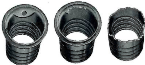
LOST LID BROKEN LUG BROKEN TOP
