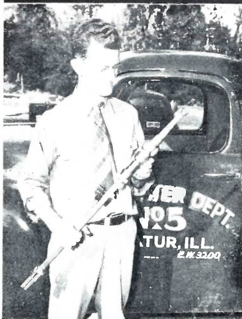
Mr. Ferguson demonstrates how the Pitometer rod meter bar is inserted in a main through a 1-inch Mueller corporation stop.
