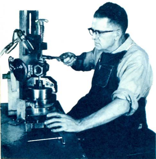
An assemblyman utilizes a torque gauge to adjust the lock nut of a Lub-O-Seal meter stop to the exact tightness.
