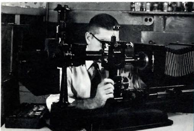
Under the extreme magnification of the Metallograph, a skilled technician inspects the microstructure of raw materials and metal in Mueller products.
