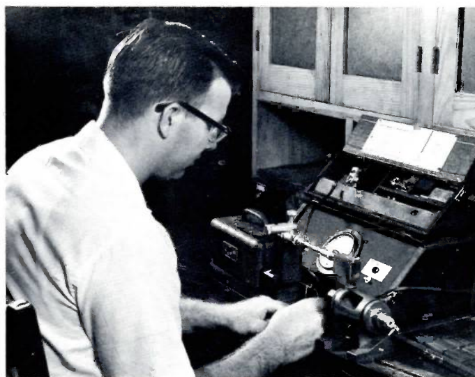
The Profilometer, a precise instrument that aids a host of inspectors in their work, reveals the surface smoothness and contours of many Mueller products.
