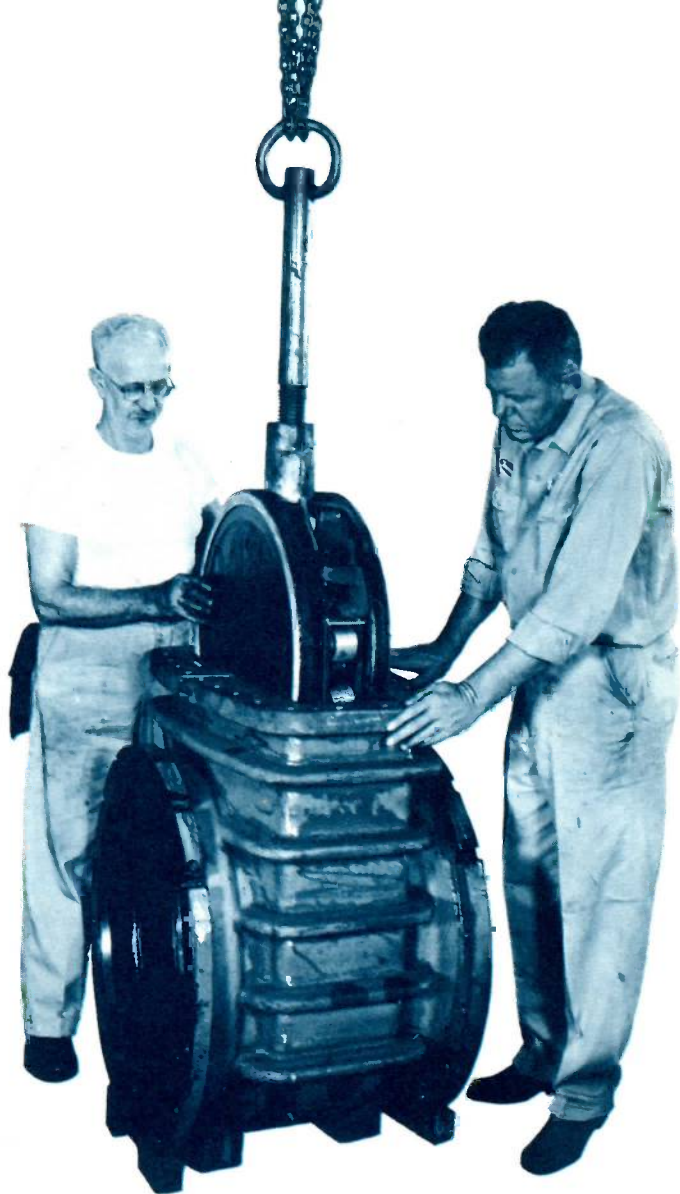
Working with great care, an experienced assemblyman expertly inserts a disc assembly into a 24" mechanical joint valve body.
