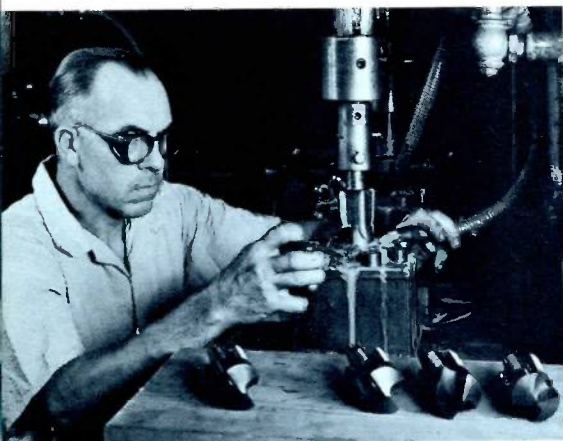
Extensive test cuts of the combined drill and tap assure a product that will give dependable performance in the field.
