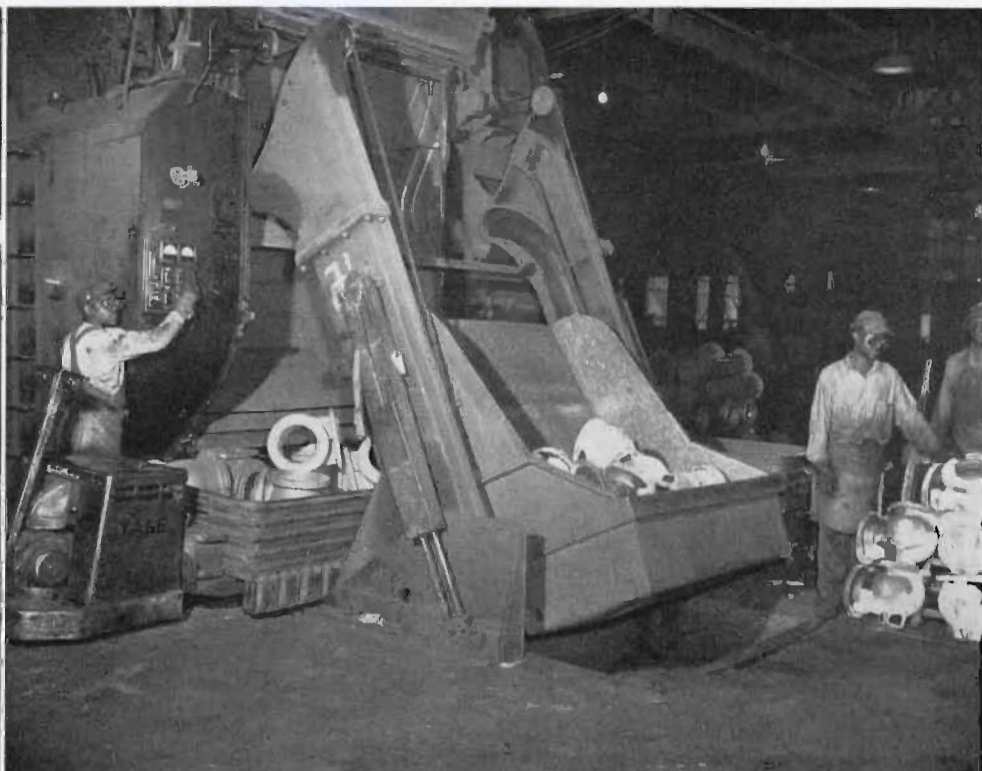
castings are run through the Pangborn cleaning machine which is shown at right. Castings in the Pangborn bucket on their way up into the machine have just left the core knock out machine. Castings in the tray have just come from inside the Pangborn. You will notice the difference in appearance of the two groups of castings. Inside the Pangborn, the cleaning operation takes place by steel shot smaller than BB shot being thrown at the castings at a terrific force while the castings are rolled over and over. The operator at the left is Jeb Thorton. The two men loading are Mitchell Love, left, and Henry McKibben. From the Pangborn, the castings are sent to the cleaning and grinding production line.
