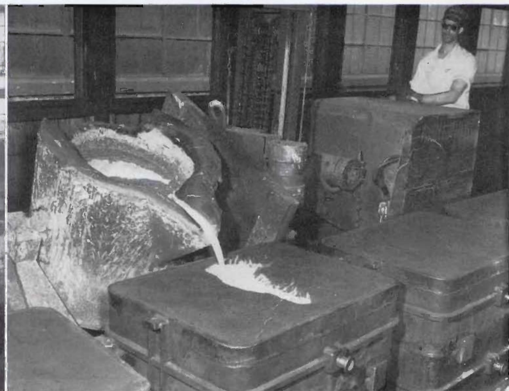
Brooks, in background, repairing cupola for next day's operations, and Jimmy Readus pouring into the ladle which is driven by Charlie Jackson. At right, Iron Pourer Chester Mason pours with a Yale fork-lift truck from a 2,000 pound capacity ladle.
