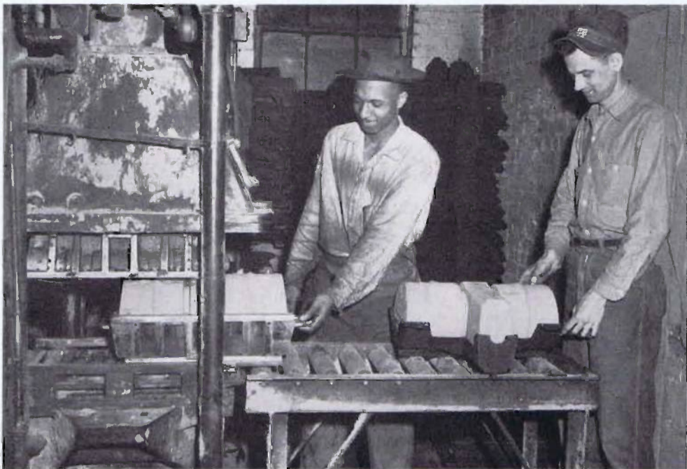
The picture at the left shows one of our large core blowers in the Chattanooga plant's Core Room. Hood Langley, right, Core Room foreman, checks the core that John Allen has just blown. This core weighs approximately 45 pounds and is blown in one piece. A blown core means that sand is blown under air pressure into the core box and forms the design of the particular core box. The sand is baked and cleaned and made ready for the molder. Blown cores weigh up to 60 pounds. Cores weighing over 60 pounds are made by hand or they are bumped. Cores made in Chattanooga's Core Room range from a few ounces to
