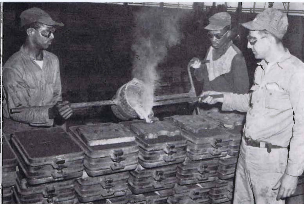
about 7,000 pounds. The core in this photo is a six-inch hub-end valve body. The photo at right shows our brass foundry which is housed in a new, well lighted and ventilated building. Though our principal items are made from cast iron, we use brass or brass lining for working parts in order to keep the movable parts from rusting. Left to right are James Brown holding the shank, LeRoy Hampton, molder pouring his own mold, and Brass Foundry Foreman Clyde Slater skimming the brass. The brass is cleaned and ground in the Brass Foundry and then sent to the Machine Shop for machining.
