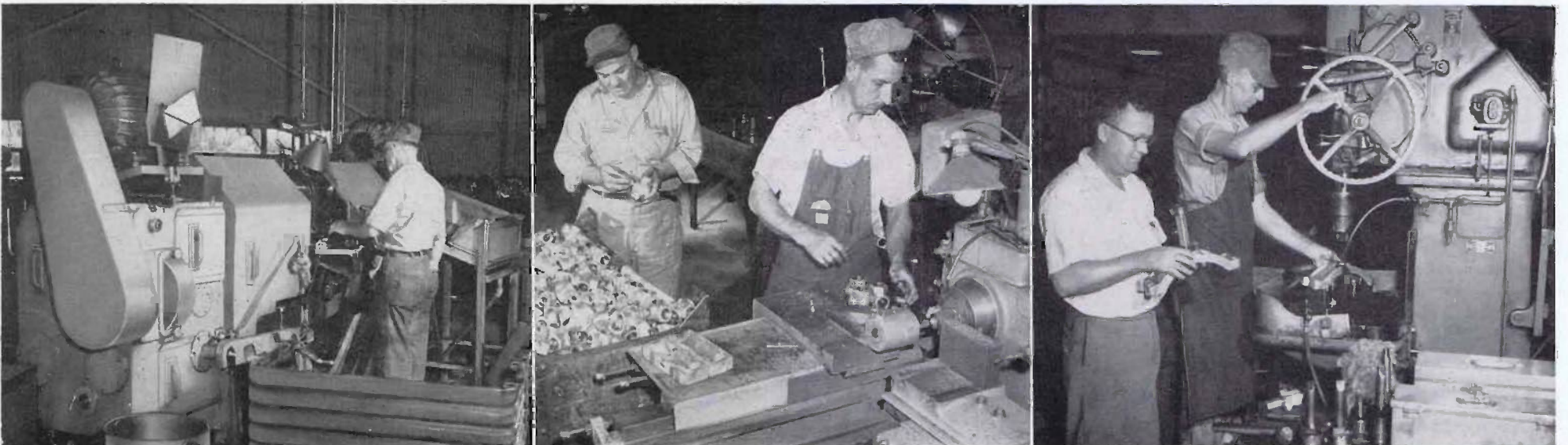
Drilling and tapping of the inlet and outlet ends of iron ground key bodies is the main purpose of this New Britain (365) automatic double end machine which is located in our Iron Machine Shop at Plant 4. The operator is William A. Hayes who has been with Mueller Co. since March 19, 1924. The center photo shows the Sun-Strand semi-automatic lathe in the Iron Machine Shop being operated by Cecil Wilson. Charles Mucray, Iron
