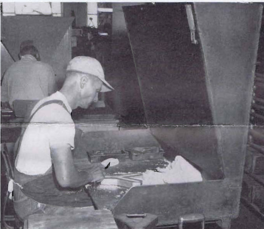
Here is a typical work bench in our Plant 4 Core Room where hand cores are made. George Anderson is leveling off sand on a core for a Y-branch connection. This core is made in halves and is one of many cores made by hand. The hand core maker naturally does not work with the speed of our modern machines, and therefore is mainly concerned with special assignments and cores for products not under a high rate of production. The hand core maker in the rear is Carl Fleischauer. At right, three operators of the Champion
