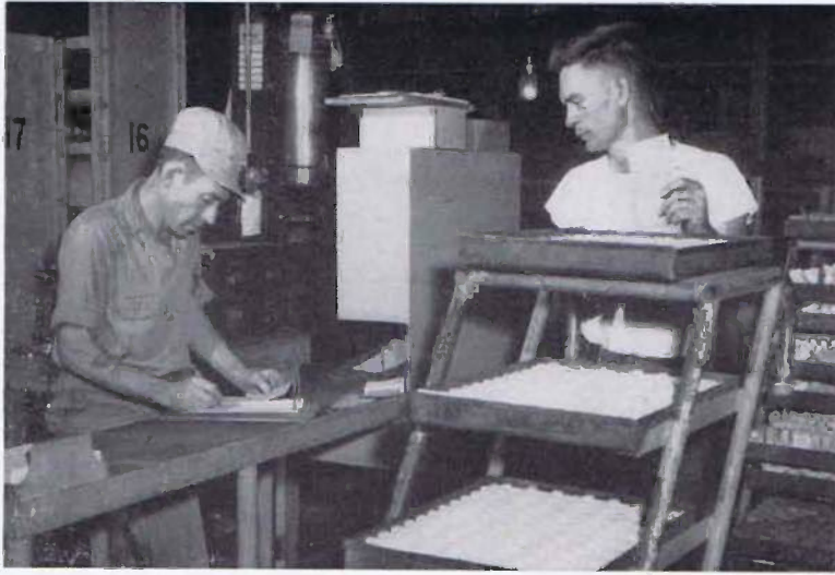
Pans of cores are delivered from the Core Room to Core Storage by roller conveyor and are placed in storage racks. As Production Control issues an order to the foundries, Edward Ellis, foundry order dispatcher, sends the proper cores to the Brass and Iron Foundries. Above, Houston Hagan, core deliver, prepares to take several pans of cores to the foundry as Ellis records the necessary data for record keeping.
