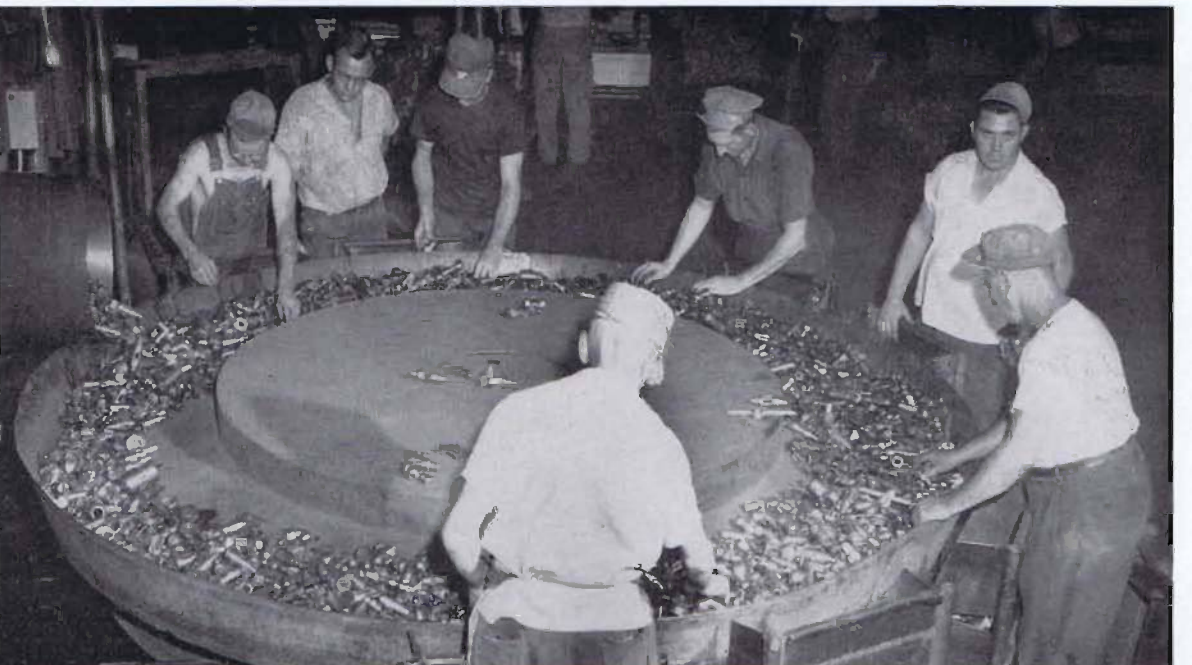
to be left for cooling. Castings are then cut off from the gates and placed in the Wheelabrator which removes adhering sand and cores. They next are placed in the Ransohoff, a large wet tumbling barrel. This gives castings a golden bronze appearance for which our products are well known. The photo at right shows castings coming from the tumbling barrel onto a round sorting table where they are sorted and placed in pans. From left around the table are Sam Jolly, Stanley Ashby, foreman; Colva Mayberry, David Isome, Pearl Kemper, George Shotton and George A. Hill.
