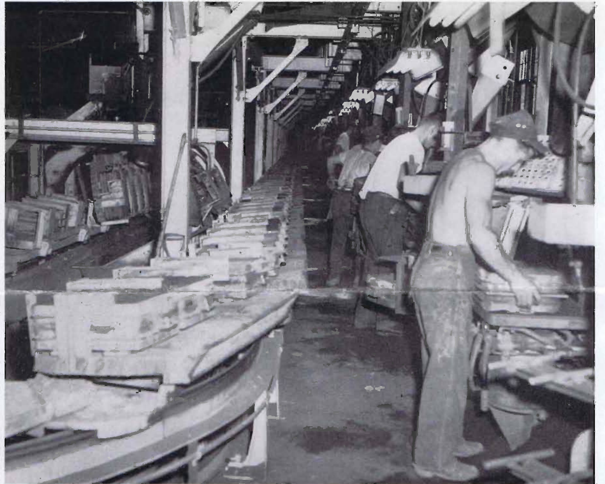
Machine molders in the Plant 4 Brass Foundry operate Milwaukee jolt-squeeze machines. The photo above shows 16 machine molders each of whom makes molds and places them on the individual cars of the train. This train indexes every six minutes, and has space for six molds for each of the 16 molders or a maximum of 96 molds for each train. While molds are being placed on one train, they are being poured on the second. The third is in a cooling section and the fourth is going through the shake out area where the sand and castings are shaken from the flasks. Note the tray of molds being dumped in the background. The first three molders in the above picture, each with assembled flask and pattern, are, front to rear, Thomas McCoy, Ronald Rutledge and James Meyers.
