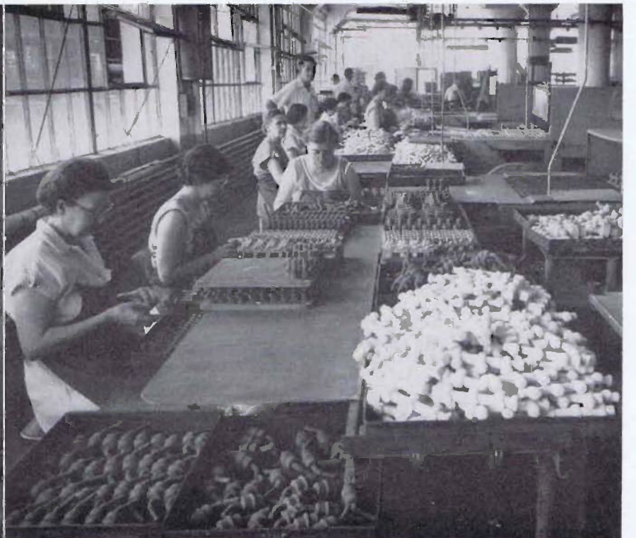
the ovens they are panned and temporarily stored on a roller skate conveyor. Cleaners and inspectors shown at work remove the cores from temporary storage to their work bench to clean and inspect them. When a pan of cores is cleaned and inspected, the pan is placed under the table on a roller conveyor which takes the cores to the core storage area. Jack Bain is Core Room foreman. Richard Ferrill is foreman trainee.
