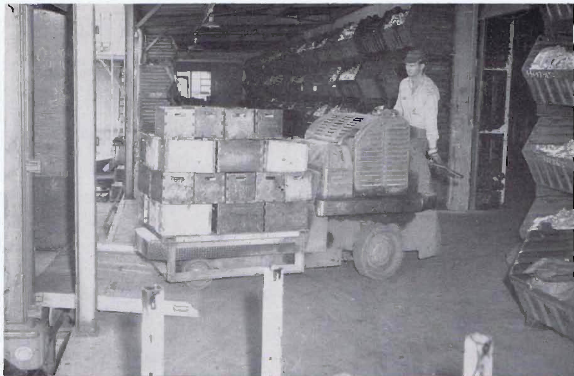
Brass castings in wooden tote boxes are being loaded into this semi-trailer truck by Benjamin Massey, Plant 4 material handler and hi-lift operator. The trailer, parked at our Plant 4 loading dock, brings the castings to Plant 1 for machining and assembly. Galvanized iron castings are stored in the background.
