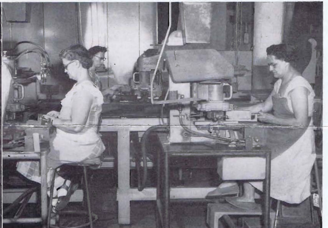
C-B-5 core blowing machines located along the 30-kilowatt dielectric core oven are blowing cores on these machines from metal boxes. Cores later are sent through the oven on wooden plates. Sand for these machines falls through a chute from the above floor. C-B-5 operators above are Fedora Tish, Dorothy Cooper and Gladys Turner. All C-B-5 operators are women.
