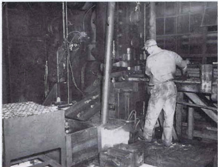
At left, the United Steel shear is shearing bar stock to forging lengths for steel tees. Operator is Fred Discher. Rotary slug heating furnace which is automatically controlled heats slugs in center photo for forging steel tees at the forging press. The furnace is being
