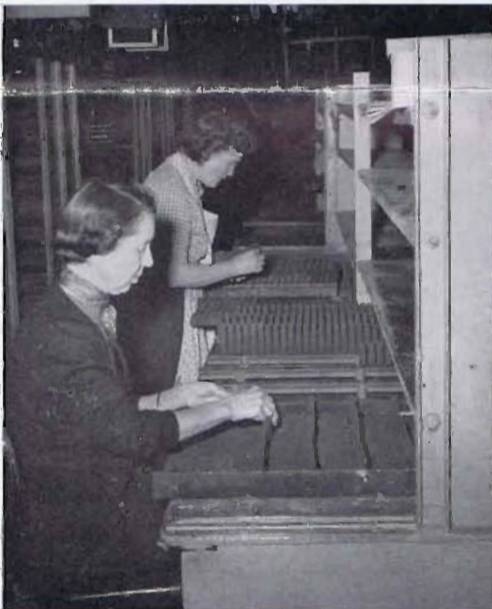
Hattie Zylicz, in foreground, and Bramlette Johnson are cleaning and inspecting cores before they go to molders. Both ladies have been with Mueller Co. eleven years. Center, Ramon Ballesteros is peening a mold. Vance Ziebarth, a twenty-year employee, at right, is
