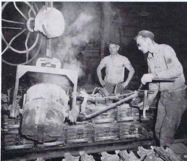
Wayne Oglesby, Core Room and Brass Foundry foreman, and a nineteen-year employee, observes molten brass being poured into molds by Chester Stinnett. In center photo, Ben Piott, an employee for twenty years, operates the cut-off machine which cuts brass castings
