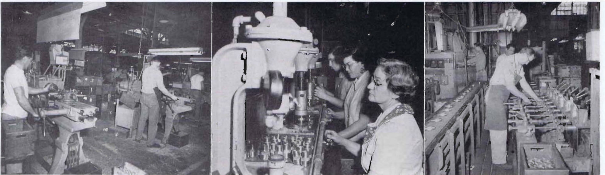
At left is a line of lathes in the Brass Machine Shop. Left to right, operators are Jimmy Musso, Mueller Co. employee for 20 years, Bernell Larsen and Jose Ortiz. Center, operators are testing spuds for cracks and foundry defects which will show up under water pressure tests. Front to back are Myrtle Baber, an 18-year employee, Donna Jolly and Ronald Young.
