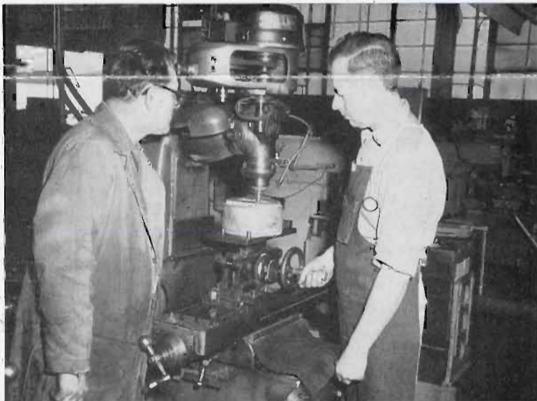
This machine is used for sinking the cavities of 1" and 3/4" steel tee dies. Left to right are Eugene Warren, tool and die foreman with the company twenty years, and Clayton Travis.
