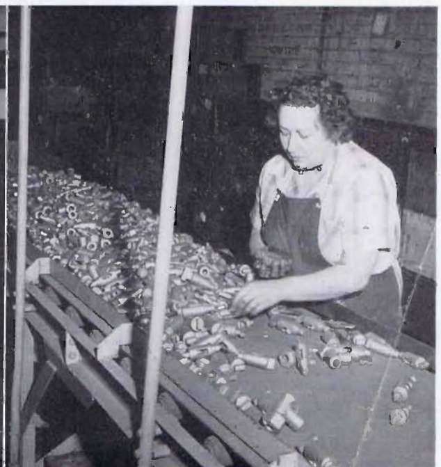
from gates. A right, Lillian Espey sorts and inspects castings after they have been cleaned at the Wheelabrator.
