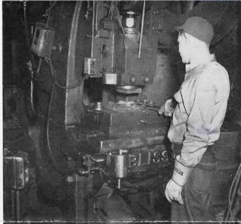
Hot steel forgings come direct from one press to this second trimming press to have the flash trimmed from the forging. Operator is Roy Estep.
