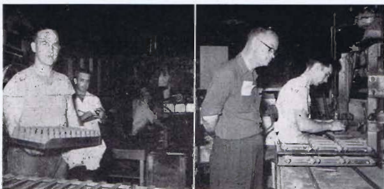
Roy Parr, oven tender, transfers cores from the coremakers to the oven in the photo at left. Ray Hazzard, Standards Department, observes the operation. The third man is Ralph Harrett at a core blowing machine. At right, George Hayward, Mueller, Limited Core Department foreman, looks over the work of John Whitley, core blower.
