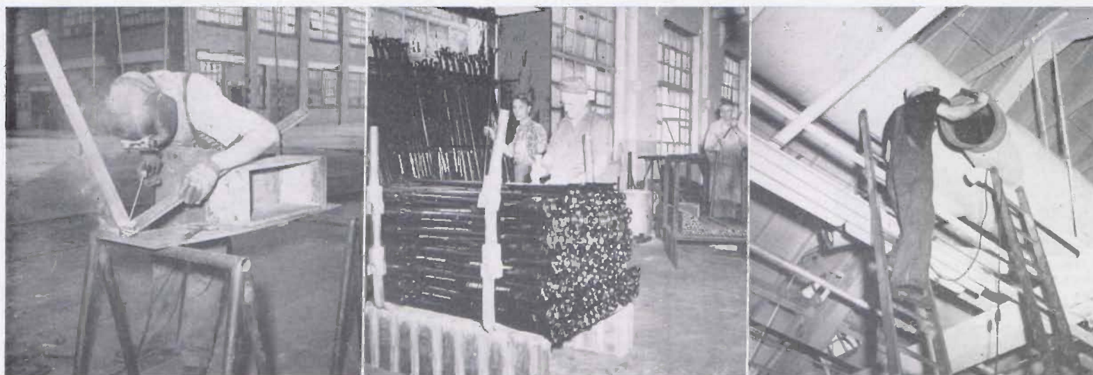
Observing the best safety measures is Harold Brown, maintenance man and welder, in the photo at left. This process is known as electric arc-welding. Three service box assemblers are shown at center. They are
