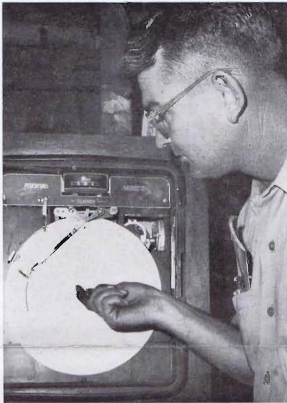
This intricate "clock" indicates to General Foreman Foundry Division Coy E. Jones the amount of winds which go into the foundry cupolas.
