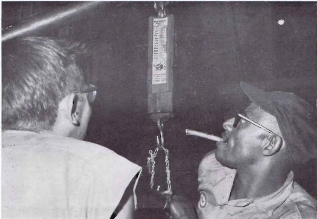
This indicator tells Machine Operator Joe Coffman (left) and his helper Jefro Hammon the amount of torque on a valve body.
