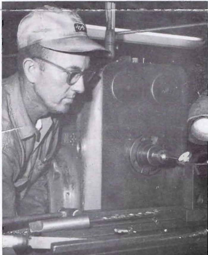
This instrument's face and hand indicate the parallelism of a block on the machine of Toolmaker Ralph Tolbert.
