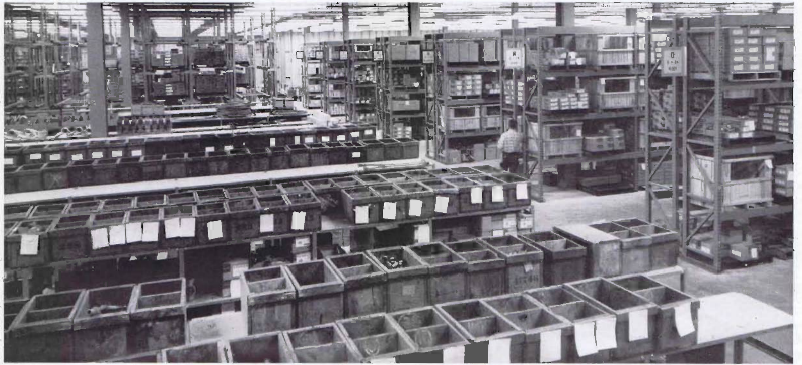
This overall view of the warehouse shows three different stocking methods. At the top, left, are the new drive-in pallet racks for high volume items. At the right are the random stock shelves and in the foreground is the low volume layout.
