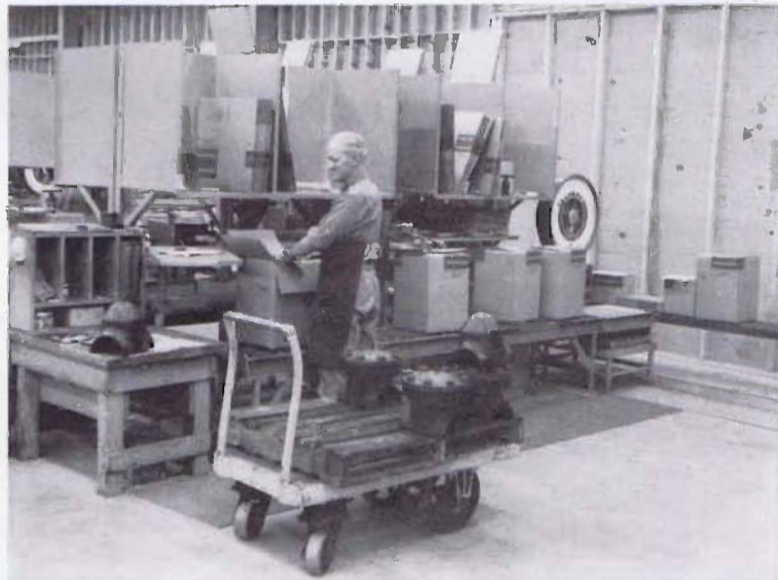
Leon Bethard checks, packs and weighs orders from this specially designed table and scale. At his work bench various sizes of cartons, packing material, and labels are available at arm's length.
