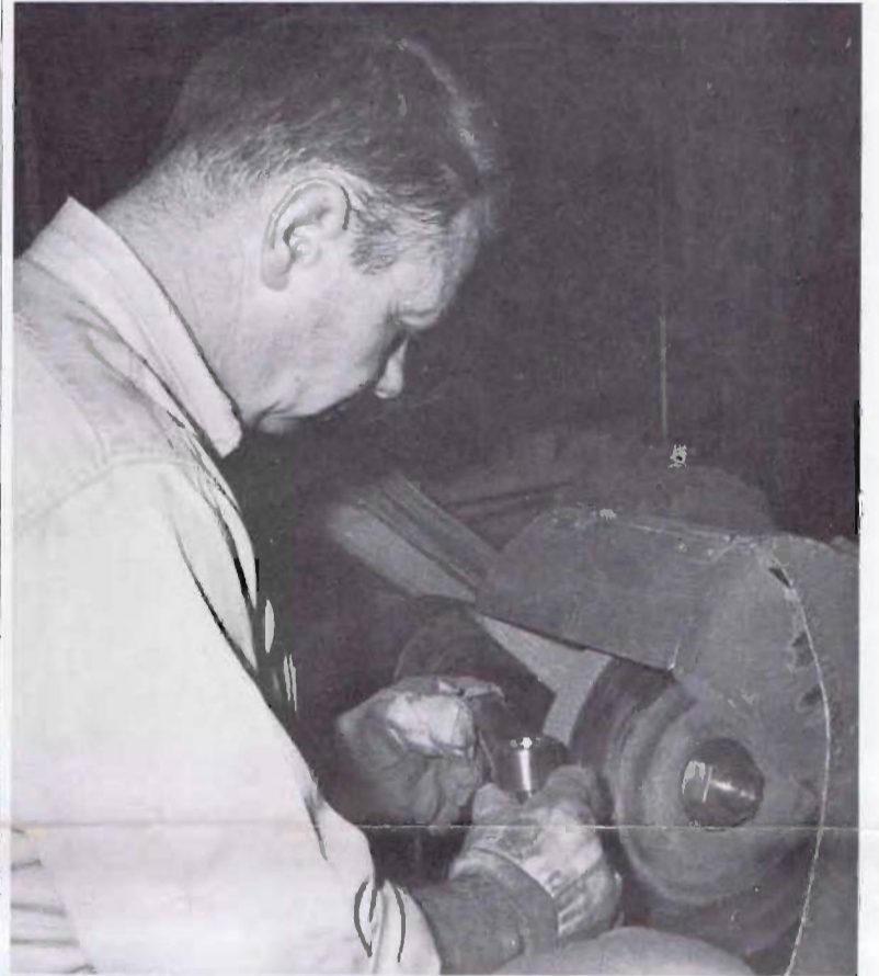
Walt Irvine demonstrates the art of polishing by working on a piece of Mueller, Limited plumbing. This skill is called the most difficult to learn of any job in the company. Carl Smith, Production Superintendent, says it takes from six to nine months to learn the proper touch.
