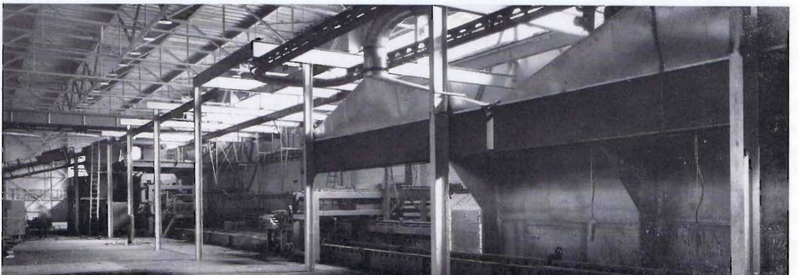
The molding machine is at the far left. The molds travel to the right into the pouring area in the foreground.
