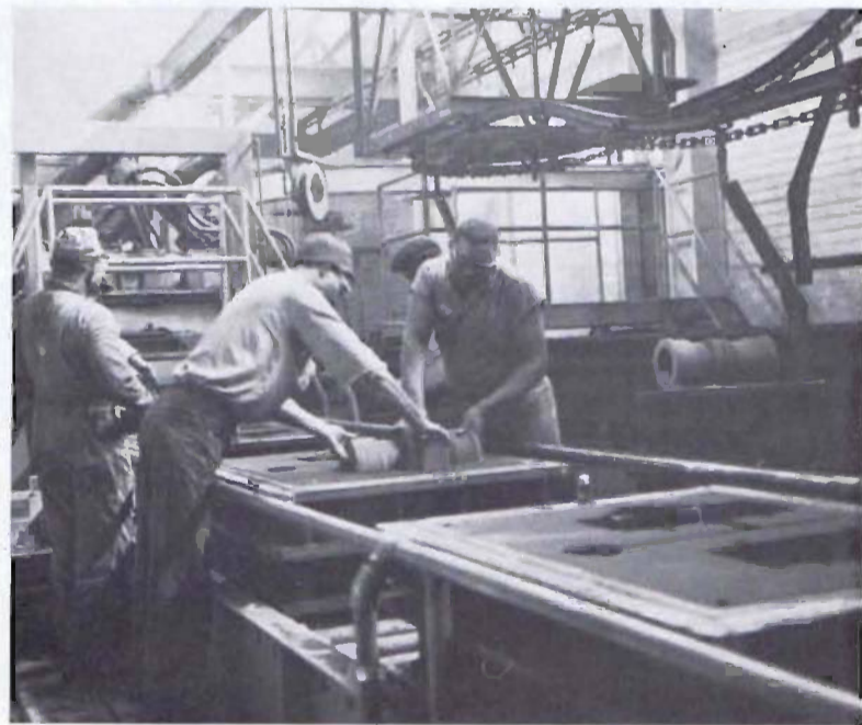
The upper photo shows the metal-pouring area on the molding machine. In the lower photo, workmen are setting cores as the molds move along the line. At the right is a conveyor that comes from the core storage area. The worker only needs to turn around to reach a new core.
