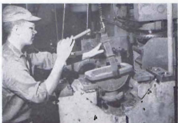
OPERATOR LOADS THE TRANSFER MACHINE.
