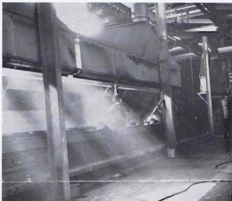
The upper photo shows the metal-pouring area on the molding machine. In the lower photo, workmen are setting cores as the molds move along the line. At the right is a conveyor that comes from the core storage area. The worker only needs to turn around to reach a new core.
