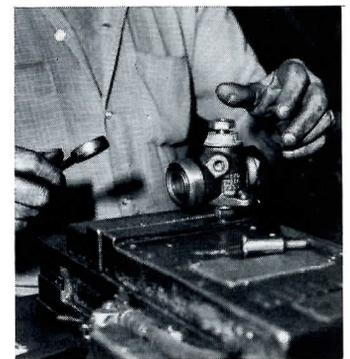
locked together with a pin, making disassembly impossible. This is why the valve is designated as Tamper Proof. The valve is filled with grease at 2,400 lbs. pressure and a plug assembled in the grease hole. Assembly continues with tightening the
