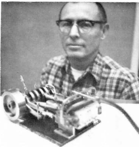
Pictured here is Jim Hudson, Dept. 80B, and his self made steam engine. This model, made in Jim's spare time, is composed of tiny, intricate valves, cylinders, etc. It presently operates on air pressure but Jim is in the process of making a boiler to complete the project.
