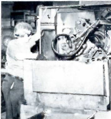
Tommy Ray Hudgins is operating the Warner and Swasey 2AC chucker machine for steel tees.
